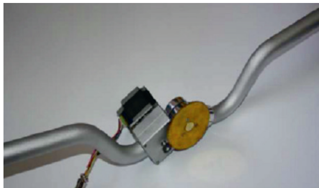
Fig. 2. Prototype of an asymmetrical upper limb exoskeleton (ULE) with a 1-side drive system
