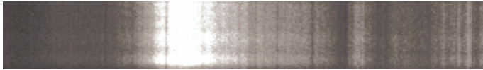
Fig. 4. Spectrum for Xe/He plasma: P_{\text{Xe}} = 1.5 \text{ MPa} , P_{\text{He}} = 0.2 \text{ MPa} , H = 1.2 \text{ mm} , \Delta x = 2 \text{ mm} and \Delta y = 800 \mu\text{m} .
