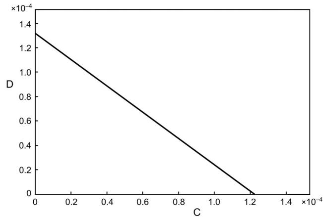
Fig. 14. Soliton pairs can be formed by having the ratio of the widths of beams as per  $r_2 = r_1(\omega_1/\omega_2)^{1/2}$ . With this width ratio of beams and parameters of Fig. 13, solutions of Eqs. (20) and (21) merge and every point of the merged line provides one soliton pair.
