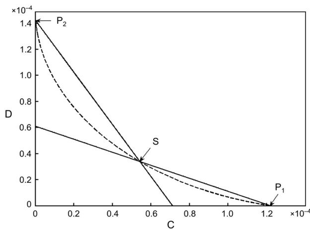
Fig. 8. With beams of the same width but different frequencies, *i.e.*,  $\omega_1 = 2.7148 \times 10^{15}$  rad/s,  $\omega_2 = 2.5148 \times 10^{15}$  rad/s, and  $r_1 = r_2 = 10 \mu\text{m}$ , Fig. 3 is modified as shown. The solitonic solution shifts towards the  $x$ -axis with  $C = 0.542 \times 10^{-4}$ ,  $D = 0.339 \times 10^{-4}$ .
