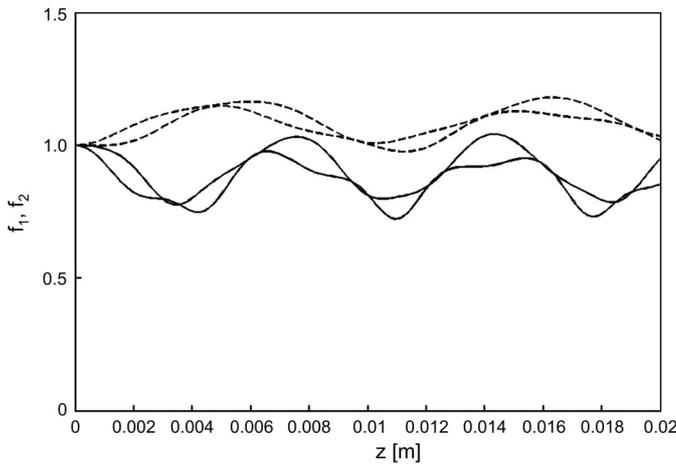
Fig. 7. Breather pair obtained from region I of Fig. 3 ( $C = 0.47 \times 10^{-5}$ ,  $D = 0.3 \times 10^{-5}$ ) is shown by dashed line and the same obtained from region II ( $C = 0.67 \times 10^{-5}$ ,  $D = 0.3 \times 10^{-5}$ ) is shown by solid line.
