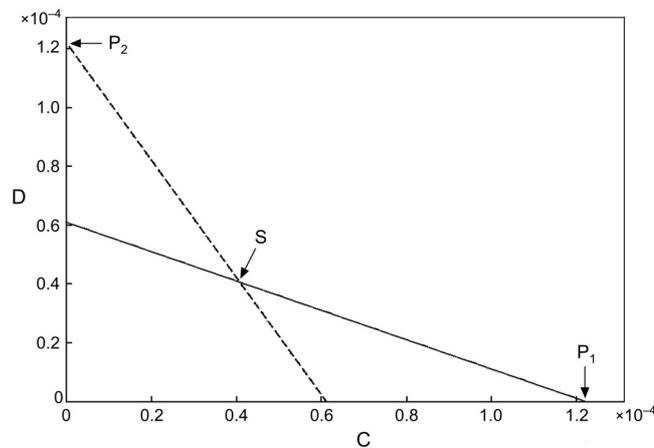
Fig. 1. Plot of  $D$  with  $C$  using Eqs. (20) and (21) for  $\kappa = 2$ ,  $\omega_1 = \omega_2 = 2.7148 \times 10^{15}$  rad/s,  $\varepsilon_{10} = \varepsilon_{20} = (1.6276)^2$ ,  $r_1 = r_2 = 10 \mu\text{m}$ .
