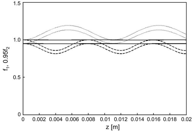
Fig. 12. If the powers of beams are chosen from a point on the existence line (of Fig. 11), both beams form a soliton pair as shown by solid lines. Here,  $0.95 \times f_2$  has been plotted to resolve  $f_1$  and  $f_2$ . If those are chosen from a point below the existence line, both beams mutually defocus and then focus, as shown by dotted lines, and if those are chosen from a point above the existence line, they mutually focus and then defocus, as shown by dashed lines.
