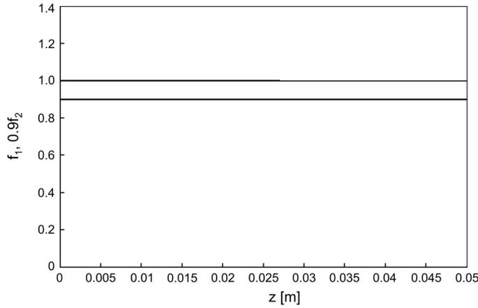
Fig. 2. Evolution of the widths of beams with the propagation distance is obtained with the parameters of Fig. 1,  $C = D = 4.0743 \times 10^{-5}$  and using Eqs. (18) and (19). The chosen widths of beams are the same, however,  $0.9 \times f_2$  has been plotted just to resolve  $f_1$  and  $f_2$ . The figure shows a soliton pair formation.
