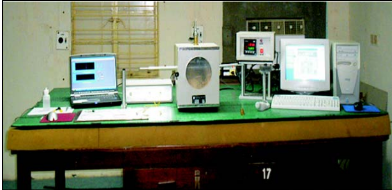
Fig. 6. Experimental setup for simultaneous application of strain and temperature.
