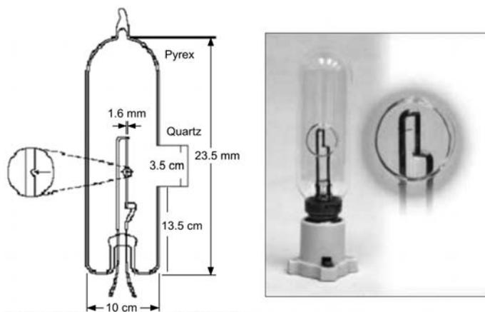
Fig. 2. Schematic drawing of the ribbon lamp [7].
