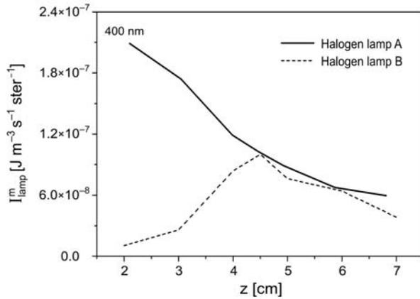
Fig. 8. Dependence of the electromagnetic radiation emitted at 400 nm by both lamp types on the distance optical system-lamp.
