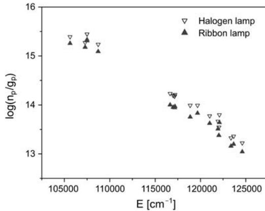
Fig. 10. Populations of the argon plasma excited levels obtained from the calibration of the optical system by two patron sources (ribbon lamp and halogen lamp). The dispersion of the populations is equal to 10%.
