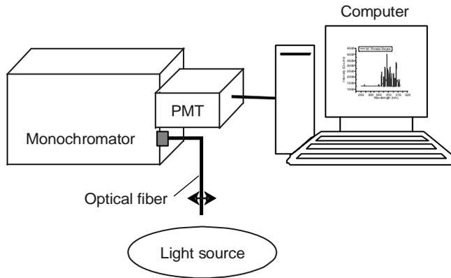
Fig. 1. Diagram of the optical system.
