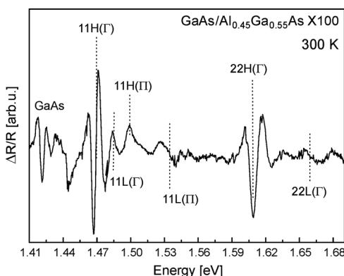
Fig. 1. Room temperature PR spectra of  $GaAs/AlGaAs$  SLs structures.
