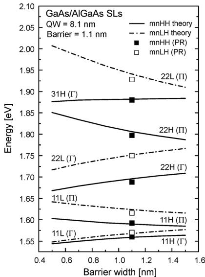
Fig. 3. The calculated energies of optical transitions for GaAs/AlGaAs SLs structures. The energies associated with heavy hole levels (solid black lines), the energies associated with light holes levels (black dashed lines). The energies taken from the analysis of PR spectra (black and white squares).
