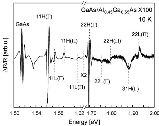
Fig. 2. The PR spectra (obtained at 10 K) of GaAs/AlGaAs SL structures.
