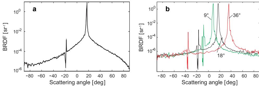
Fig. 5. Test BRDF of silicon wafer using measurement system: BRDF data of Ag-coated reflector at a 9° angle of incidence (a), BRDF data of polished silicon wafer at 9°, 18°, and 36° angles of incidence (b).
