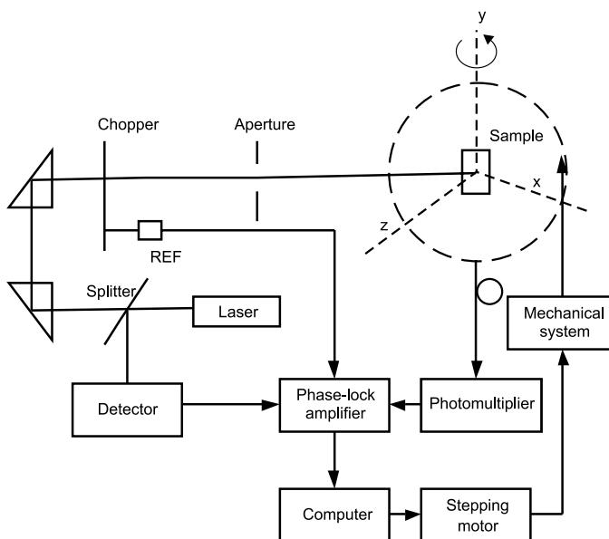
Fig. 3. Arrangement of measurement system.
