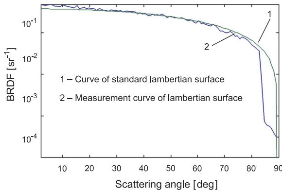
Fig. 4. Calibration curve of measurement system.
