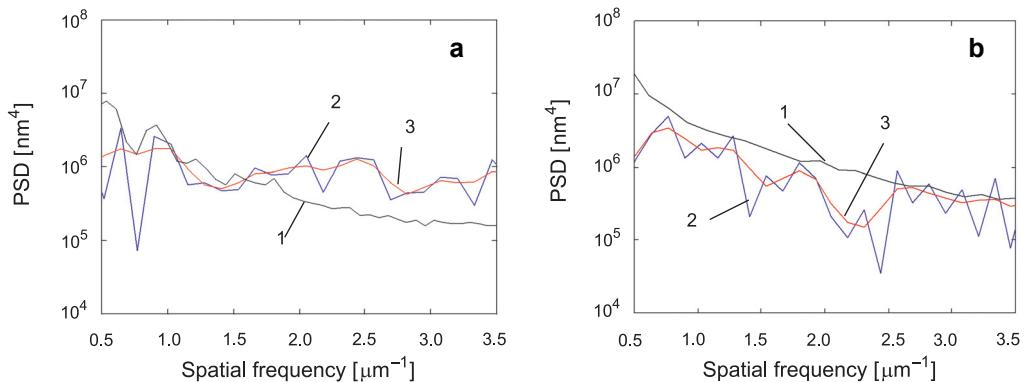
Fig. 7. PSD of two surfaces using different test methods: PSD curve of silicon wafer (a), PSD curve of Ag-coated reflector (b).
