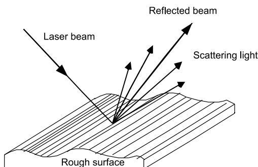
Fig. 1. Laser light scattering from rough surface.
