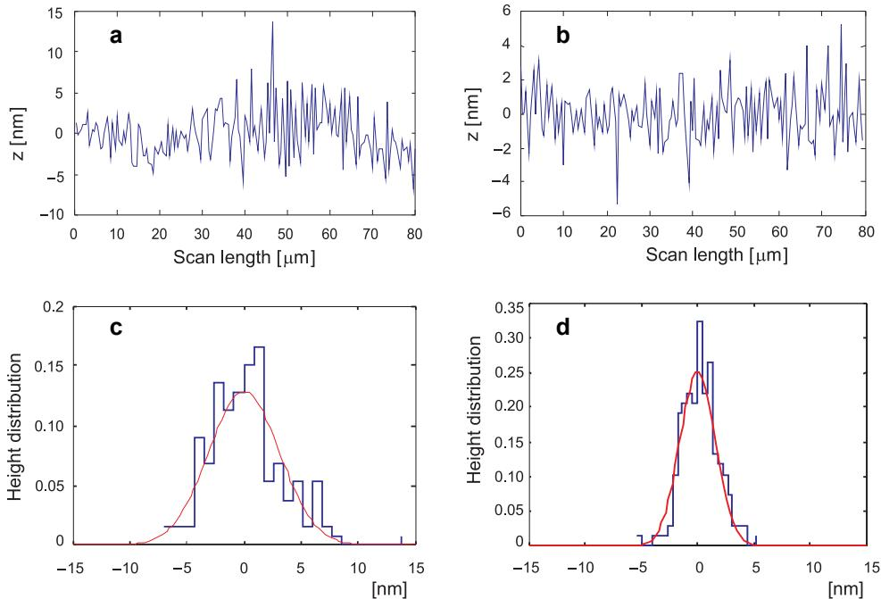
Fig. 6. Tested roughness data of silicon wafer and Ag-coated reflector using profile meter: surface profiler of silicon wafer (a), surface profiler of Ag-coated reflector (b), height distribution function of silicon wafer (c), height distribution function of Ag-coated reflector (d).
