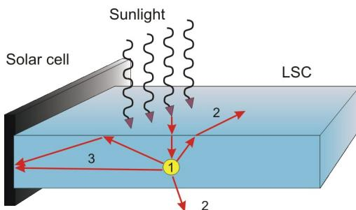
Fig. 1. Schematic of a luminescent solar concentrator. 1 – nanopowder Nd,Yb:YAG, Nb,Yb:GGG or Nd,Yb:YO that absorbs and emits photons; 2 – photons emitted outside the region of total internal reflection (losses); 3 – photons transported to the solar cell.
