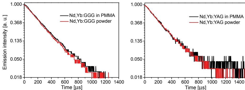
Fig. 7. Room temperature emission decays of Nd,Yb:GGG (a) and Nd,Yb:YAG (b) powders as well as PMMA plate measured under 976 nm excitation.
