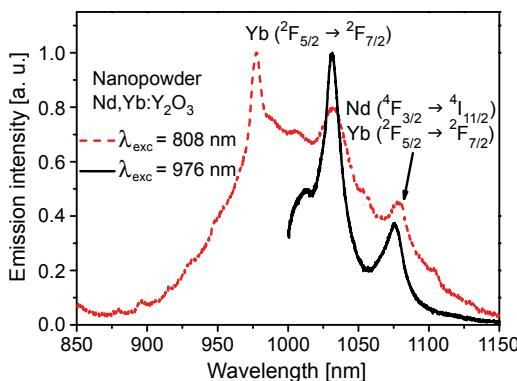
Fig. 6. Emission spectra of Nd,Yb:YO powder obtained under 808 nm and 976 nm excitation.
