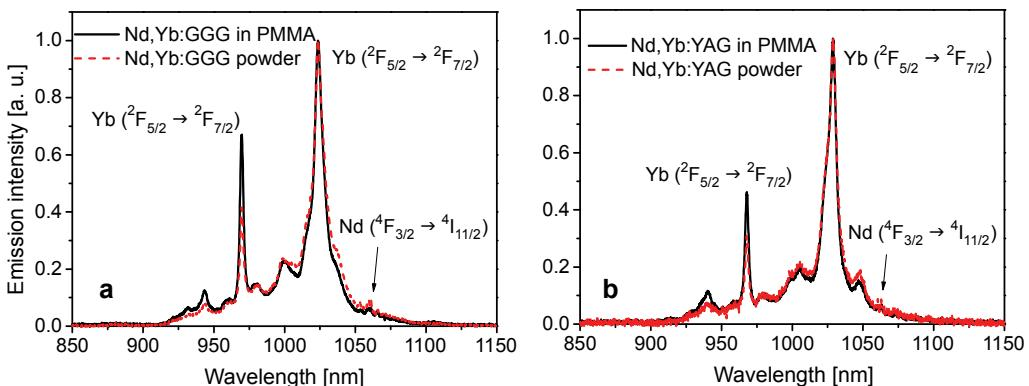
Fig. 3. Emission spectra of Nd,Yb:GGG (a) and Nd,Yb:YAG (b) powders as well as PMMA plate measured under 808 nm excitation.
