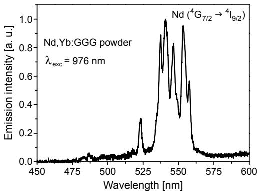
Fig. 5. Up-conversion fluorescence spectra of Nd,Yb:GGG excited at 976 nm.
