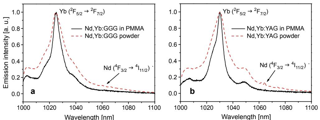
Fig. 4. Emission spectra of Nd,Yb:GGG (a) and Nd,Yb:YAG (b) powders as well as PMMA plate measured under 976 nm excitation.
