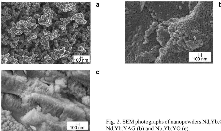
Fig. 2. SEM photographs of nanopowders Nd,Yb:GGG (a), Nd,Yb:YAG (b) and Nb,Yb:YO (c).
