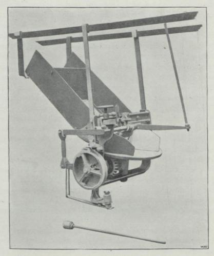
Fig. 73.—Suspended Challenge Ore-Feeder and Hopper. Rod and Rubber Buffer lying at bottom.
