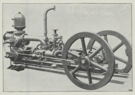
Fig. 61.—Riedler Pump in use at the Geldenhuis Deep. Compound engine driven by compressed air, the pump being placed at the bottom of the vertical shaft at a depth of about 600 feet. Speed at this head 150 revolutions per minute. Plungers 3\frac{1}{8} in. and 5\frac{1}{4} in. with a 16-in. stroke. Air cylinders 10 in. and 14 in. with a 16-in. stroke. Air pressure, 70-75 lbs. per square inch.
