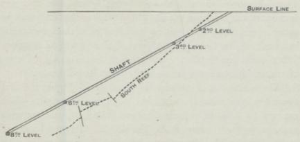
Fig. 55.—Section through the Central Shaft of the City and Suburban Mine.
