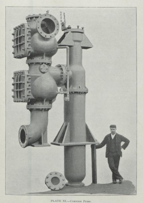
Diameter of ram, 14 inches; stroke, 10 feet. Greatest working speed, 10 strokes per minute.
