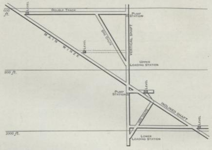
Fig. 6o.—Proposed Arrangement for reducing number of Stations at one of the South Simmer and Jack Shafts.
