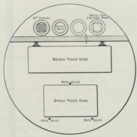
Fig. 52.—Section of Round Shaft at the New Primrose.
