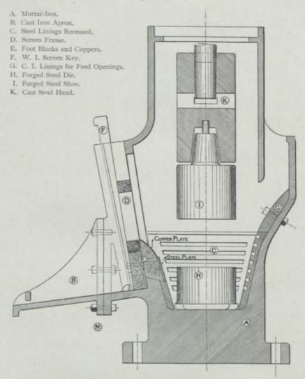
Fig. 76.—Section of the Mortar used at New Crossus Mine, showing Stamp Head, Shoe, Die, and other parts.
