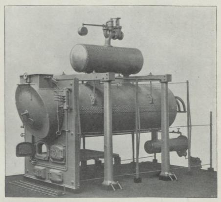
Fig. 65.—Horizontal Multi-tubular Under-fired Boiler. A type largely used in the Rand. Diameter, 66 inches; length, 16 feet; heating surface, 1500 square feet; grate surface, 33 square feet; total weight, 15 tons; nominal horse-power, 125; evaporation of water, 4500 lbs. per hour.
