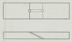
Fig. 77. - False Bottom for worn-down Dies,
