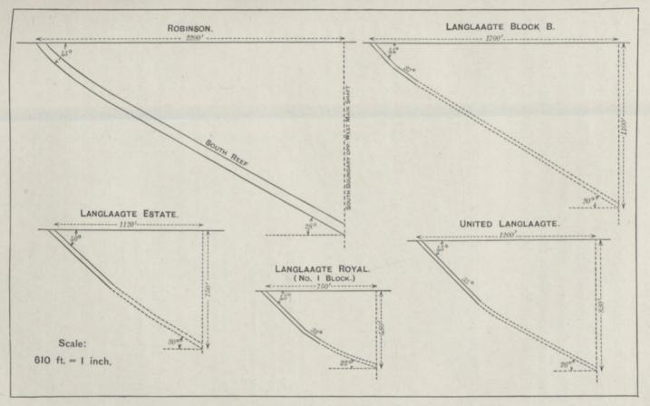
Fig. 49.—Diagrams illustrating the Decrease of the Angle of Dip in Depth—Continued.
