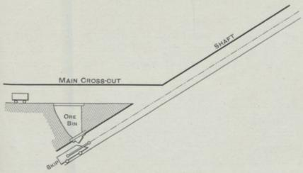
Fig. 58.—Arrangement for loading Skips.
