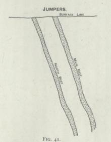
lie the payable ore-bodies, which are taken out in one big stope. They consist of two main bodies. The uppermost of these (Middle Reef) is distinguished by a slaty parting on the foot-wall. It consists of some 15 to 20 inches of pay ore. In the western part of the mine it is split up into two small leaders separated by a seam of sandstone. Of these the foot-wall leader, although small, is very rich.
