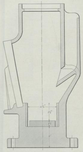
Fig. 75.—Mortar-Box at the City and Suburban.
