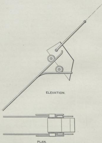
Fig. 62-Plan and Section of a Self-dumping Skip.
