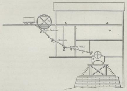
FIG. 66.—Diagrammatic Section of the Sorting-House at the Roodepoort United Main Reef Company's Mine.
