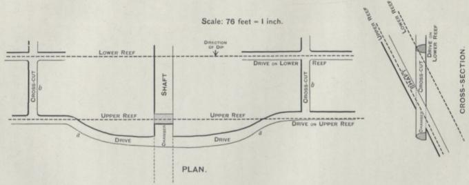
Fig. 56.—Plan of Levels and Cross-cuts.
