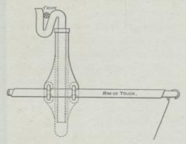
FIG. 68.—Jockey used in Endless Rope-haulage.
