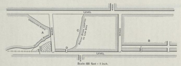
Fig. 57.—Diagram showing Methods of Stoping.
