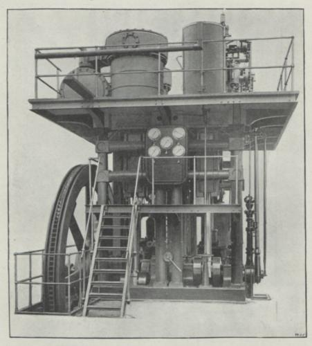
FIG. 64.—The "BURLY" COMPRESSOR in use at the Nourse Deep. Indicated horse-power, 350; revolutions per minute, 70; steam pressure, 120 lbs. Compound steam cylinders with Corliss valve gear. Compound air cylinders with inter cooler steam cylinders both jacketed with live steam.
