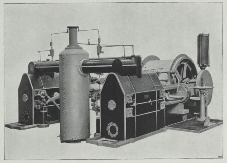
PLATE XII.—WINDING ENGINE, 20" × 48", IN USE AT THE JUMPERS DEEP.
