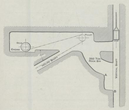
Fig. 59.—Proposed Arrangement for working Deep Level Mines.
