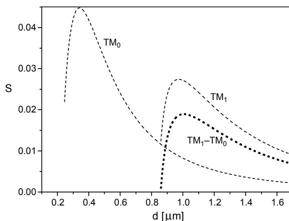
Fig. 4. Sensitivities as a function of the thickness of the waveguide layer at TM polarization.
