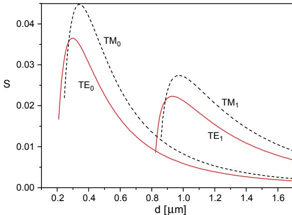
Fig. 2. Sensitivities as a function of the thickness of the waveguide layer.
