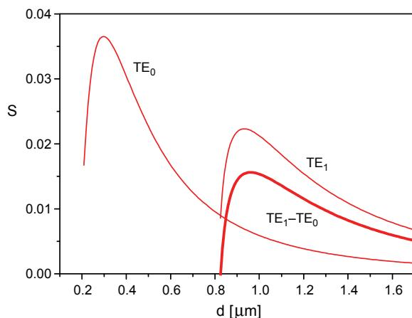
Fig. 3. Sensitivities as a function of the thickness of the waveguide layer at TE polarization.
