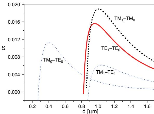
Fig. 5. Sensitivities as a function of the thickness of the waveguide layer concerning various pairs of modes.
