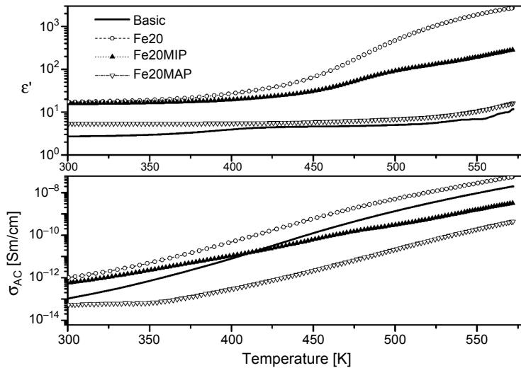
Fig. 2. Temperature dependences of dielectric permittivity  $\epsilon'$  and conductivity  $\sigma_{AC}$  for microporous (Fe20MIP), macroporous (Fe20MAP) magnetic glasses, for two-phase Fe20 glass and basic (nonporous) alkali borosilicate glass at 5 Hz.
