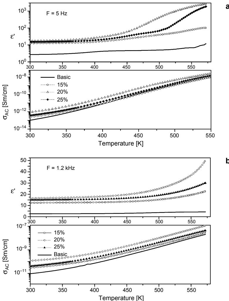
Fig. 1. Temperature dependences of dielectric permittivity  $\epsilon'$  (top) and AC conductivity  $\sigma_{AC}$  (bottom) for the initial two-phase magnetic glasses with different concentrations of iron oxide and for the basic nonporous glasses (without iron oxide) – solid lines at 5 Hz (a) and 1.2 kHz (b).
