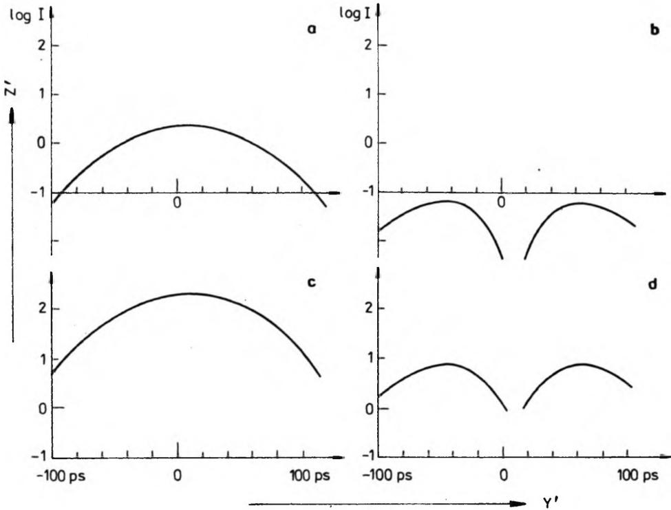
Fig. 2. Time-dependent intensity for a diffracted 50 ps-pulse at four positions in the image plane  $B(Y', Z')$ : **a**  $-(Y', Z') = (0, A)$ , **b**  $-(Y', Z') = (A, A)$ , **c**  $-(Y', Z') = (0, 0)$ , **d**  $-(Y', Z') = (A, 0)$ ,  $A = 2.5 \times 10^{-4}$  cm
