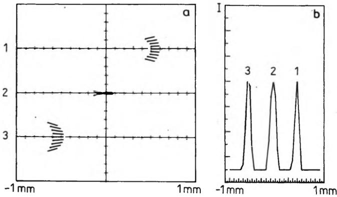
Fig. 6. Spot diagrams (a) and slit-integrated intensities (b) for meridional coma:  $1-t = -30$  ps,  $2-t = 40$  ps,  $3-t = 100$  ps
