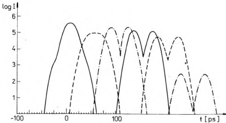
Fig. 3. Pulse shape at six different image positions, from left to right:  $Y' = 0, 2.5, 5, 7.5, 10$  and  $50 \mu\text{m}$ ,  $Z' = 0$
