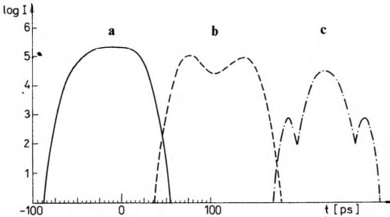
Fig. 4. Double and triple pulses by grating diffraction
