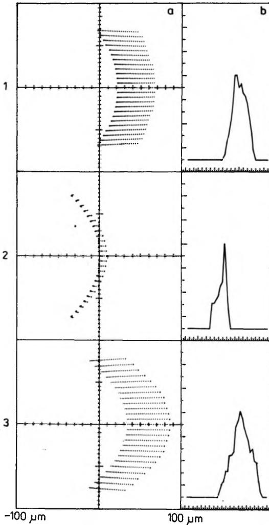
Fig. 5. Movement of the focus: **a** - spot diagrams for different times, **b** - intensities derived from ray tracings. 1 -  $t = -120$  ps, 2 -  $t = 0$ , 3 -  $t = 120$  ps
