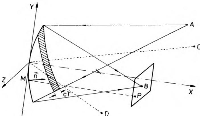
Fig. 1. Diffraction of a short light pulse by a corrected holographic concave grating
