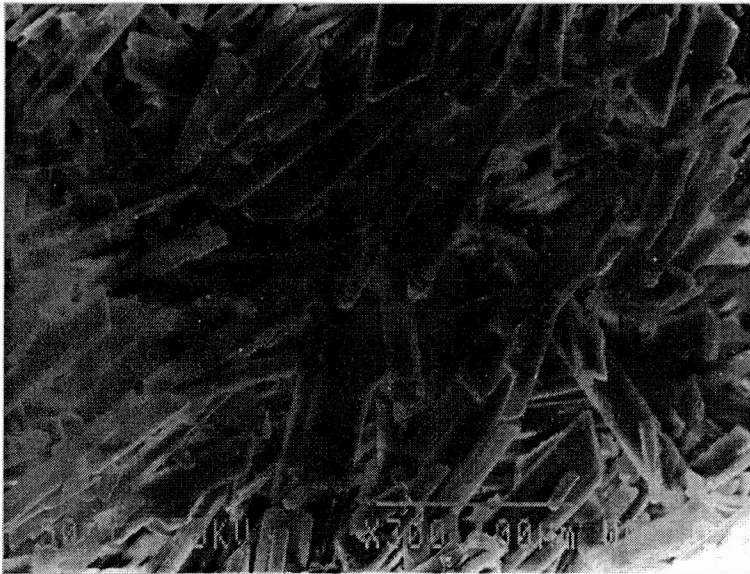
Fig. 7. SEM photograph of crystalline structure of phosphogypsum taken from plant's pipe ( \times 1,000 )
