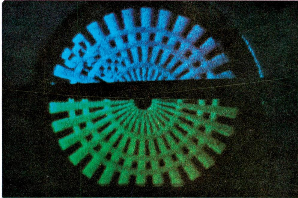
Phot. An image of a two-colour image reconstructed with a white light from the rainbow hologram
