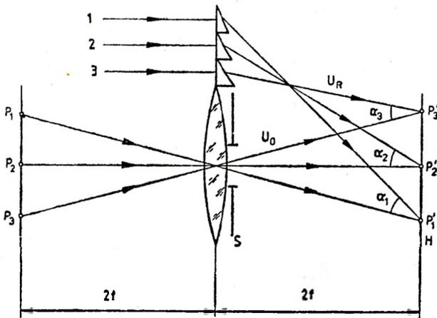
Fig. 1. Optical system for production of the rainbow holograms by using three different reference beams (1, 2, 3)
