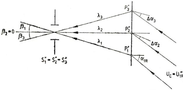
Fig. 3. The reconstruction of the rainbow hologram using collimated beam of white light
