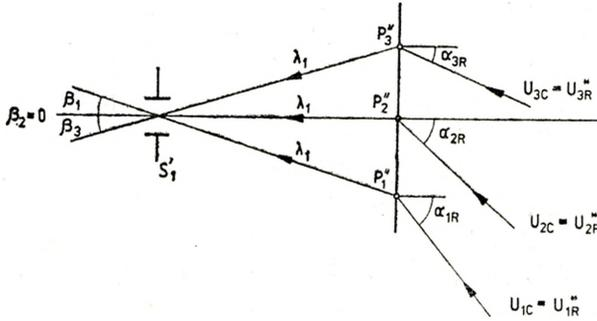
Fig. 2. The reconstruction of the rainbow hologram by using beams conjugated with the respective reference beams
