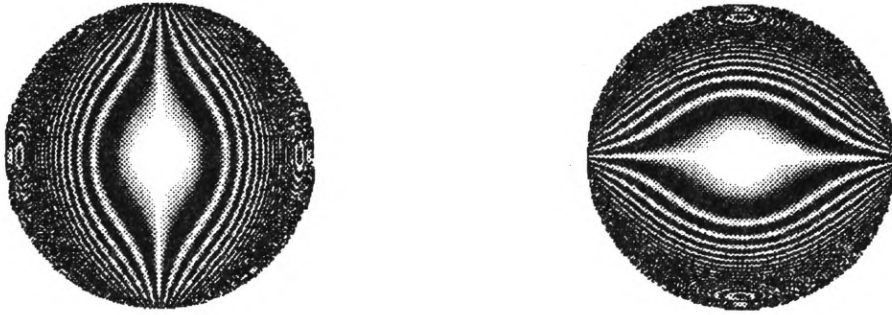
Fig. 13. x and y -deflectograms for simulation 4. The specimen is aspherical (symmetrical ellipsoid), the rotation function R_1(\varphi) is given by: R_1(\varphi) = \text{const} = 7.80 mm, the aperture diameter is 30 mm, p/d = 2 \cdot 10^{-4} , R_2 = 7.87 mm, R_0 = 7.86 mm. The deflectograms appear smaller because of different radius of curvature on the optical axis (Fig. 7b). The low density fringe spacing in the outer region (horizontal in the x -deflectogram) indicates locations where the ellipsoid intersects the sphere with radius R_0 .
