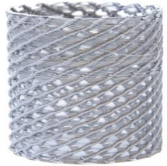
Fig. 13. 18 ribs with 120°, V_{rib} : 400 mm/min, V_{cyl} : 1600 mm/min
