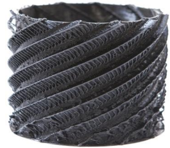
Fig. 6. 18 ribs with 120°, extrusion 5 mm, V_{rib} : 400 mm/min, V_{cyl} : 800 mm/min
