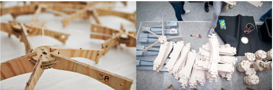
Fig. 3. (Left) Connectors and nodes before quick impregnation (photo author: Mateusz Olczyk). (Right) Detail of node in 1:5 scale prototype (photo author: Mateusz Olczyk)
