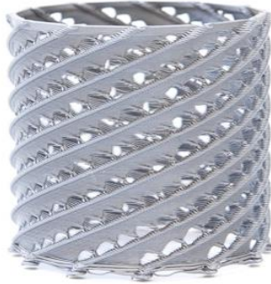
Fig. 12. 12 ribs with 120°, V_{rib} : 400 mm/min, V_{cyl} : 1600 mm/min
