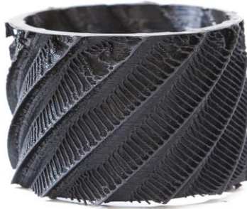
Fig. 5. 12 ribs with 60°, extrusion 5 mm, V_{rib} : 400mm/min, V_{cyl} : 800 mm/min
