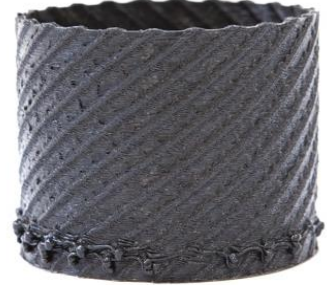
Fig. 3. 24 ribs with 120°, V_{rib} : 400 mm/min, V_{cyl} : 800 mm/min
