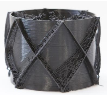
Fig. 8. 6 ribs with 60° and - 60°, extrusion 5 mm, V_{rib} : 400 mm/min, V_{cyl} : 800 mm/min
