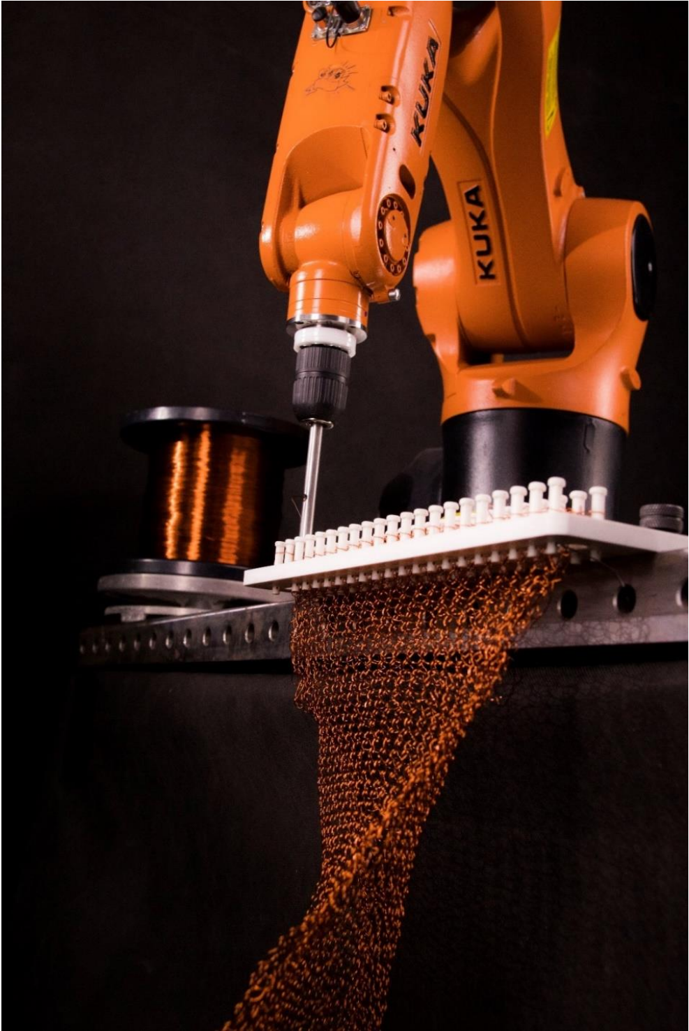
Fig. 1. The process of knitting a copper structure by a robot. Photo: M. Mojsiejuk
