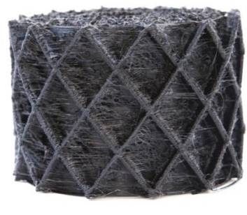
Fig. 10. 12 ribs with 60° and - 60°, extrusion 5 mm, V_{rib} : 400 mm/min, V_{cyl} : 800 mm/min
