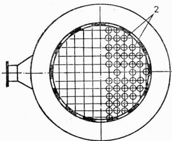
Fig. 5. Block of multicyclones of diameter of 15 m
