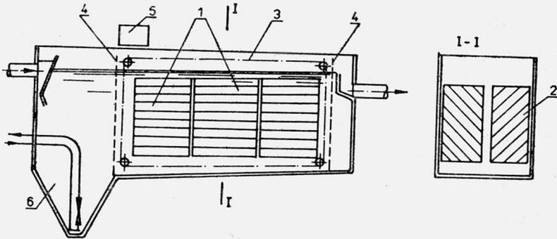
Fig. 2. Multi-tier settlers operating in transversal mode
