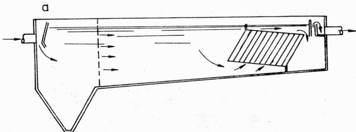
Fig. 4. Flow diagram of the existing settling tanks equipped with blocks of parallel plates
