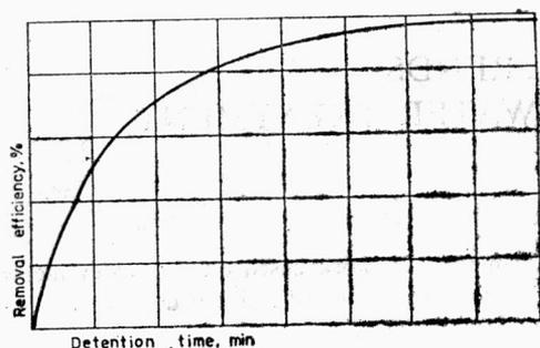
Fig. 1. Kinetics of wastewater sedimentation
