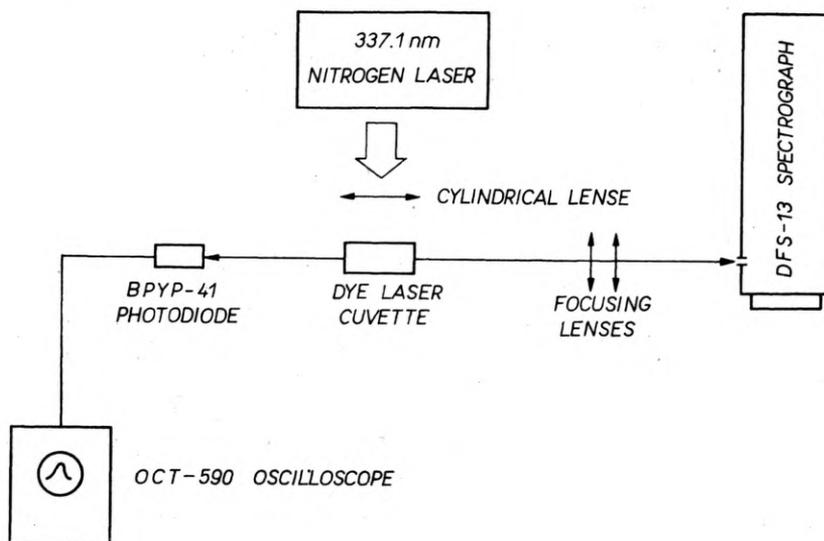
Fig. 2. Experimental setup
