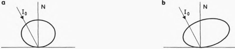
Fig. 1. Angular characteristics: a – SE, b – BSE. ( I_0 – primary beam, N – normal to the specimen surface)
