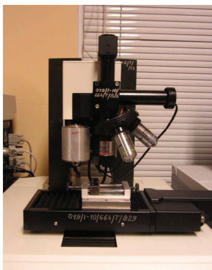
Rys. 4.20. Nanoindenter TTX-NHT, CSM Instruments
