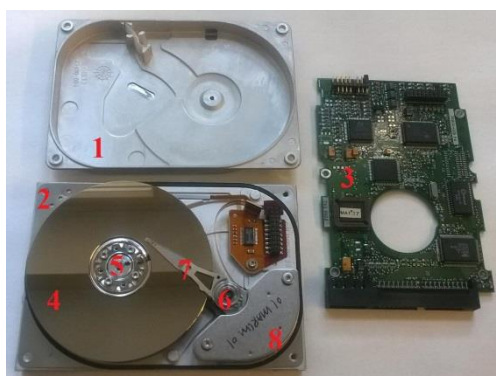
Fig. 1. Hard disk from CONNER company: Particular elements: 1 – top cover; 2 – mounting chassis; 3 – electronics card; 4 – platter; 5 – spindle; 6 – read/write head; 7 – head arm, 8 – actuator
