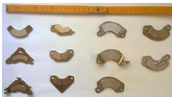
Fig. 3. The examples of magnets assembly of actuator from different hard disk drives (HDDs)
