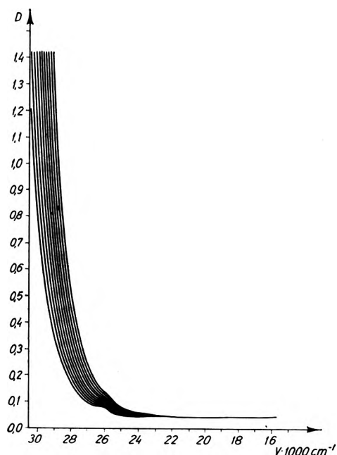
Fig. 4. The shift of the absorption edge in the F5 glass within the 20°C - 220°C temperature range
