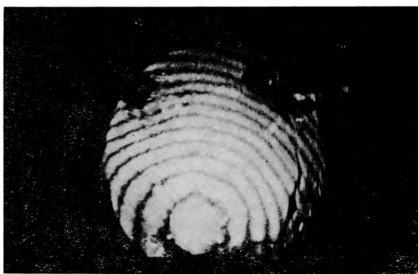
Fig. 12. An image reconstructed from the hologram. An interferogram of a pill with deposited electrodes to which a 1500 V-voltage is applied
