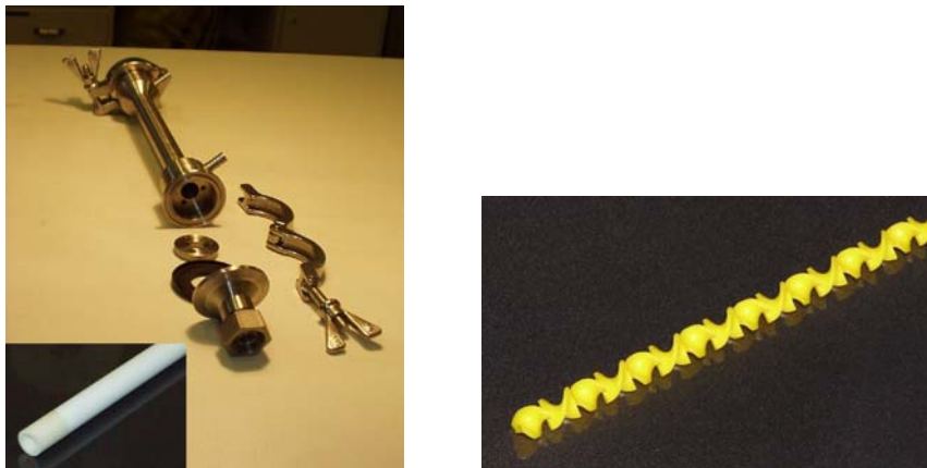
Fig. 1. The membrane with its housing and the static mixer
