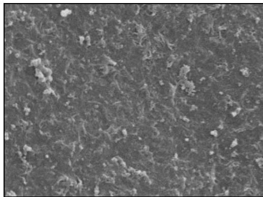
Fig. 10. SEM image of surface of new pipeline made of PE after biofilm removal
