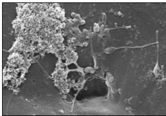
Fig. 8. SEM image of biofilm developed on surface of new pipeline made of PP
