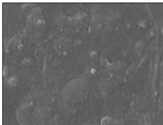
Fig. 12. SEM image of surface of new pipeline made of PP after biofilm removal
