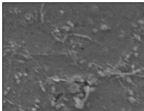
Fig. 5. SEM image of biofilm developed on surface of new pipeline made of PVC
