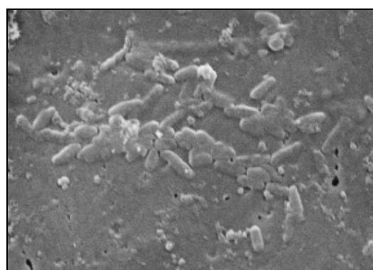
Fig. 7. SEM image of biofilm developed on surface of new pipeline made of PB
