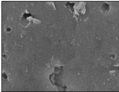
Fig. 9. SEM image of surface of new pipeline made of PVC after biofilm removal
