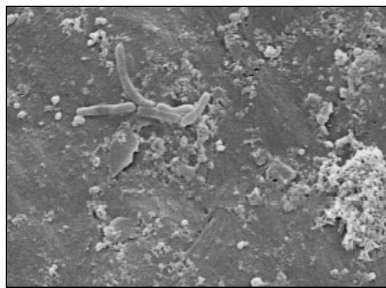
Fig. 11. SEM image of surface of new pipeline made of PB after biofilm removal
