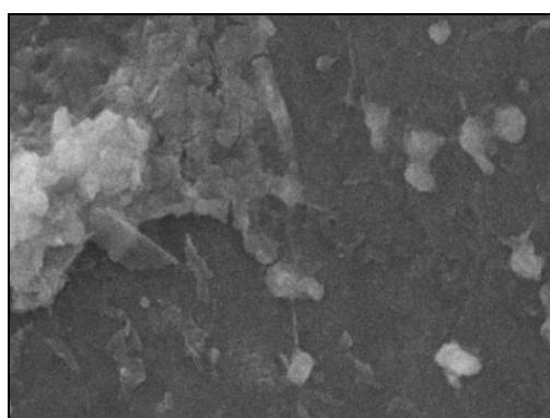
Fig. 6. SEM image of biofilm developed on surface of new pipeline made of PE
