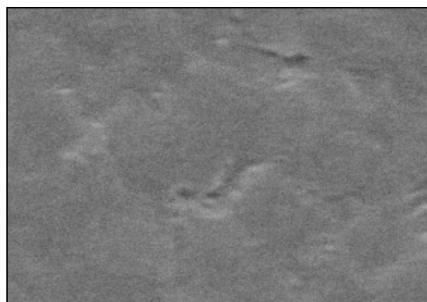
Fig. 2. SEM image of surface of new pipeline made of PE (magnification of 6 000 $\times$ )
