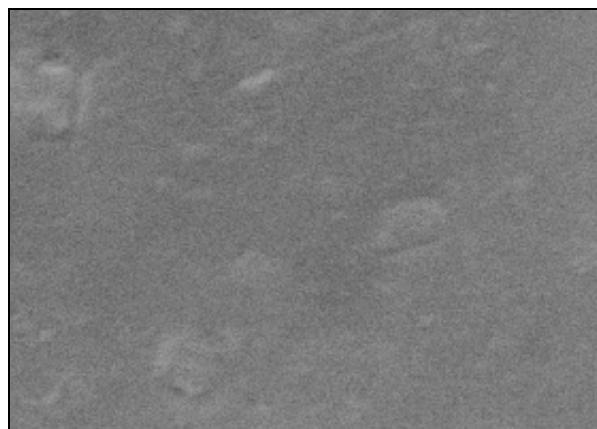
Fig. 1. SEM image of surface of new pipeline made of PVC (magnification of 6 000 $\times$ )
