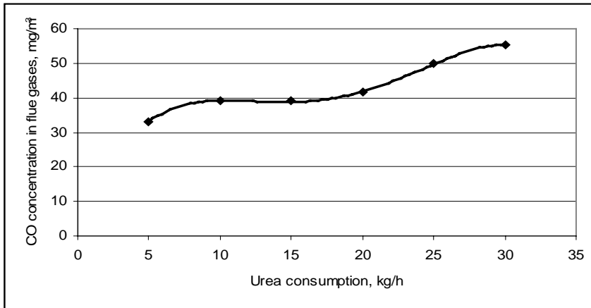
Fig. 6. CO concentration in cleaned flue gases versus urea consumption
