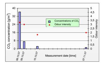
Fig. 2. Average concentration of  $CO_2$  and odour intensity in the air above the surface of the screenings storage yard
