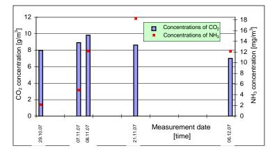
Fig. 7. Average concentration of CO<sub>2</sub> and NH<sub>3</sub> in the air in the poultry house
