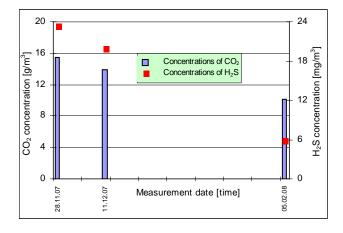
Fig. 5. Concentration of CO<sub>2</sub> and H<sub>2</sub>S in the leachate catch pit at the waste dumping site
