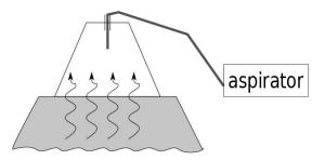
Fig. 1. Schematic diagram of the air sampling by flux chamber from a surface-based source
