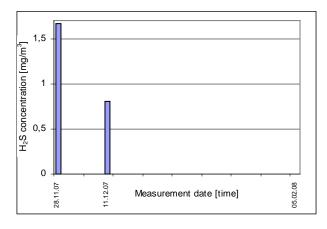
Fig. 6. Concentration of H<sub>2</sub>S in the ventilation well at the waste dumping site
