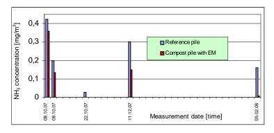
Fig. 4. Average concentration of NH<sub>3</sub> in the air above the surface of the compost piles
