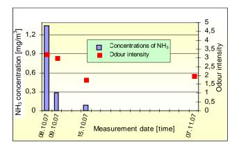
Fig. 3. Average concentration of NH<sub>3</sub> and odour intensity in the air above the surface of the screenings storage yard
