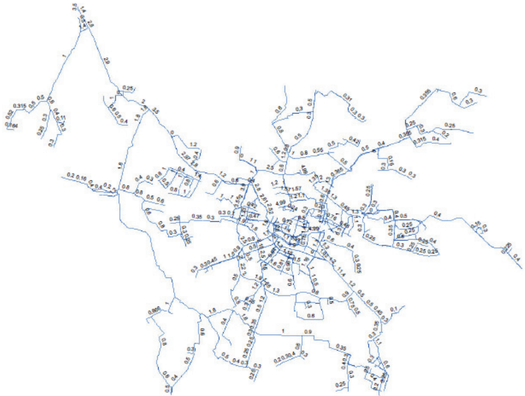
Fig. 1. The framework of sewerage system in Wrocław [12]
