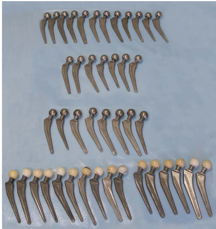
Fig. 4.1.1. The examined hip implants retrieved during revision surgeries mainly for aseptic loosening.
