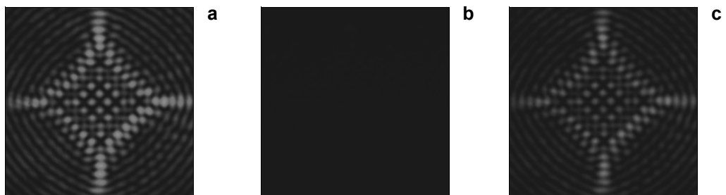
Fig. 7. Experimental intensity distributions when the polarization is parallel to the c -axis ( \varphi_p = \varphi_c = 0^\circ ): x -component ( \varphi_a = 0^\circ ) – a , y -component ( \varphi_a = 90^\circ ) – b , and x - and y -component ( \varphi_a = 45^\circ ) – c .
