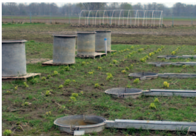
Phot. 6. Evaporimeter pots prepared for installation at the measurement sites in the Agro- and Hydrometeorological Observatory Wrocław-Swojec
