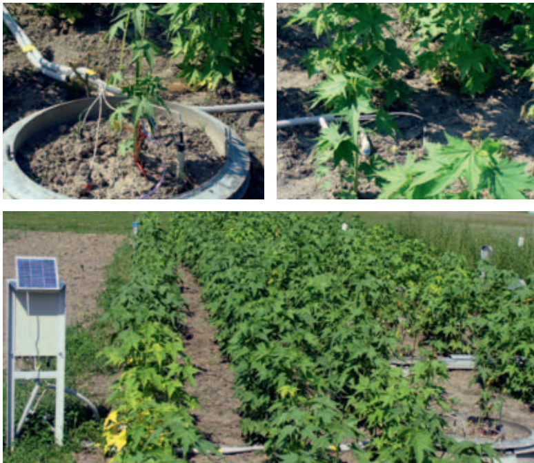
Phot. 11. TDR probes installed in a plot and an evaporimeter under Virginia mallow
