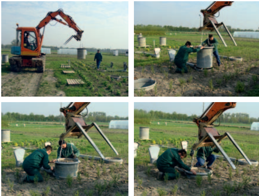
Phot. 8. Installation of evaporimeter at a measurement site in the Agro- and Hydrometeorological Observatory Wrocław-Swojec
