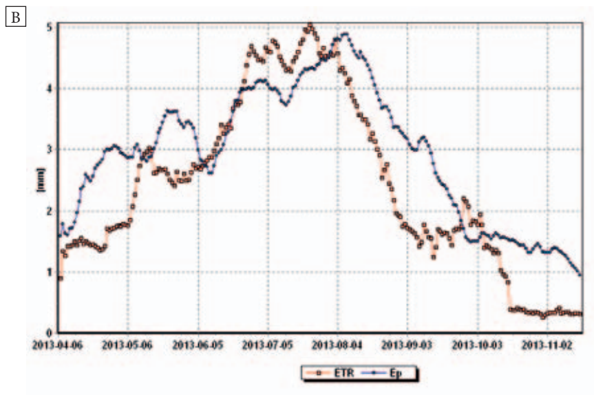
Fig. 21. Empirical input data from 2013, evaporimeter No. 1: ETR – evapotranspiration, Ep – input data calculated with EVAPO A – Basket willow ( Salix viminalis ), B – Virginia mallow ( Sida hermafrodita Rusby) Source: own elaboration
