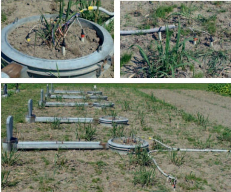
Phot. 10. TDR probes installed in a plot and an evaporimeter under Miscanthus sinensis giganteus
