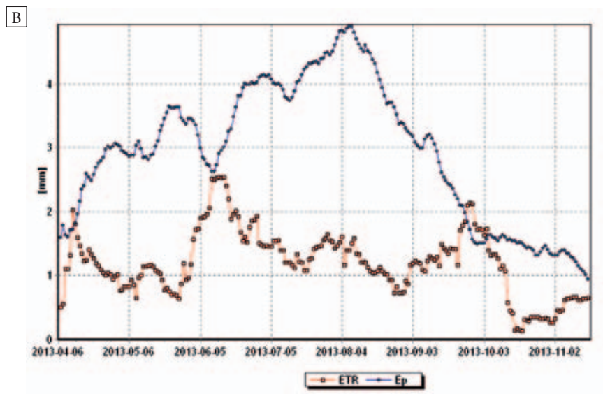
Fig. 23. Empirical input data from 2013, evaporimeter No. 1: ETR – evapotranspiration, Ep – input data calculated with EVAPO A – Giant miscanthus grass ( Miscanthus x giganteus ) B – Jerusalem artichoke ( Helianthus tuberosus ) Source: own elaboration
