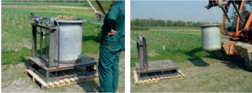
Phot. 7. Measurement of evaporimeter mass prior to its installation at a measurement site in the Agro- and Hydrometeorological Observatory Wrocław-Swojec
