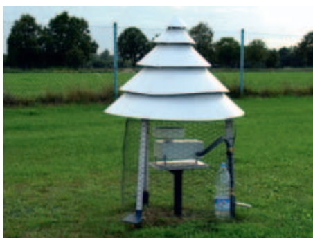
Phot. 3. Evaporimeter EWP 992 on a measurement site at the Agro- and Hydrometeorological Observatory Wrocław-Swojec
