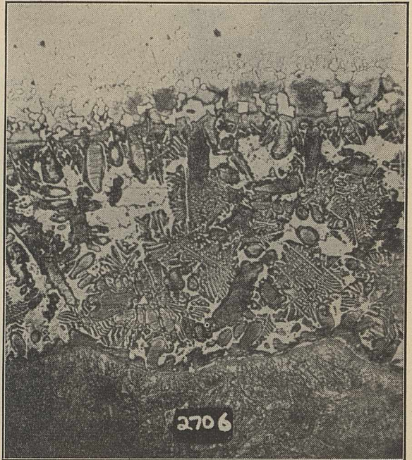
Section across junction of high-speed steel tip and plain carbon steel tool shank using Stalweld Powder as bonding material. (x 500) Taken on 'Wratten' Metallographic plate through a yellow filter.
