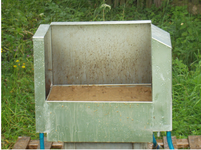
Fot. 4.6. Skrzynia pomiarowa do oznaczania rozbryzgu w warunkach terenowych (fot. autor) Phot. 4.6. Splash box device for soil splash measurements in natural conditions (phot. author)
