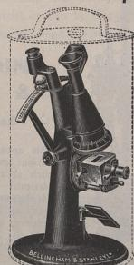
A Polarising Eyepiece for the examination of doubly refracting fatty materials can be provided, and also an Electric Lamp Attachment for back illumination of dark or opaque materials.
