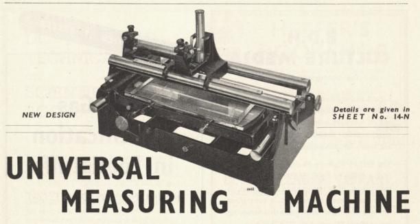
For the accurate measurement of Records, and of opaque or translucent objects
