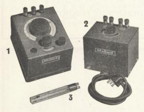
**CONDUCTIVITY MEASURING EQUIPMENT.** This apparatus consists of Measuring Bridge Type GM 4140 (1), 1,000 cycle Oscillator Type GM 4260 (2) and Conductivity Cell Type GM 4221 (3). The apparatus is highly sensitive and covers a range of conductivity between 1.0 reciprocal ohm to greater than 10 reciprocal megohms.
