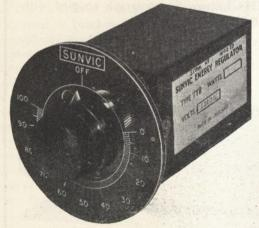
The Energy Regulator as an industrial controller has only recently begun to take its proper place among industrial equipment. The Energy Regulator replaces a variable resistance and will control up to 30 amps A.C. or D.C. It will keep the energy input constant, independent of mains voltage fluctuations, at any setting between no load and full load and will do this without the energy dissipation inevitable with resistance control. It is particularly valuable for industrial furnaces and hotplates.
