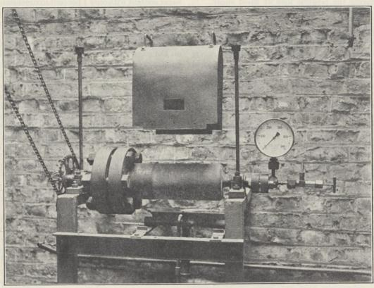
FIG. 1. Bergius 2-litre converter. From Fuel Research Technical Paper No. 42. Crown copyright reserved.
