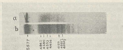
FIG. 1. Spectrum of (a) zodiacal light plus night sky; total exposure, 27 hours; (b) night sky; exposure, 75 hours.
