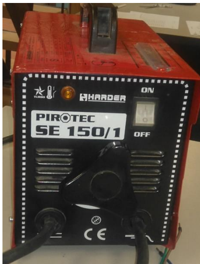
Rys. 7. Transformator spawalniczy firmy HARDER umieszczony w KMNiPE Politechniki Wrocławskiej Fig. 7. Welding transformer created by HARDER, placed in Cathedral of Electrical Machines Drives and Measurements
