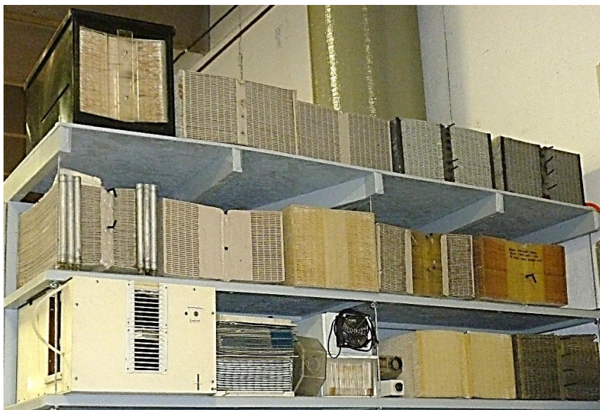
Fig. 1.19. Different versions of the cross-flow M-Cycle HMXs which were tested over the years (author's photograph).
