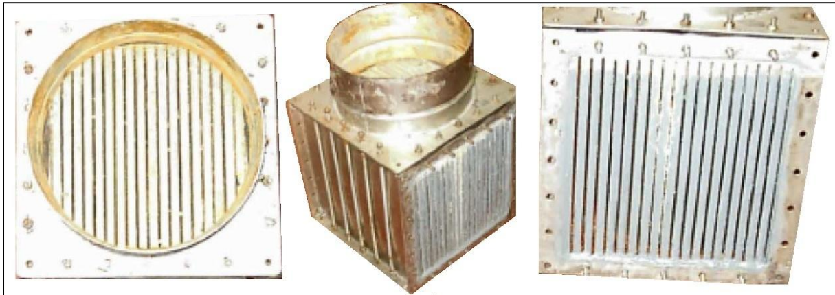
Fig. B1. Photograph of the exchanger used by Martinez et al. [68].
