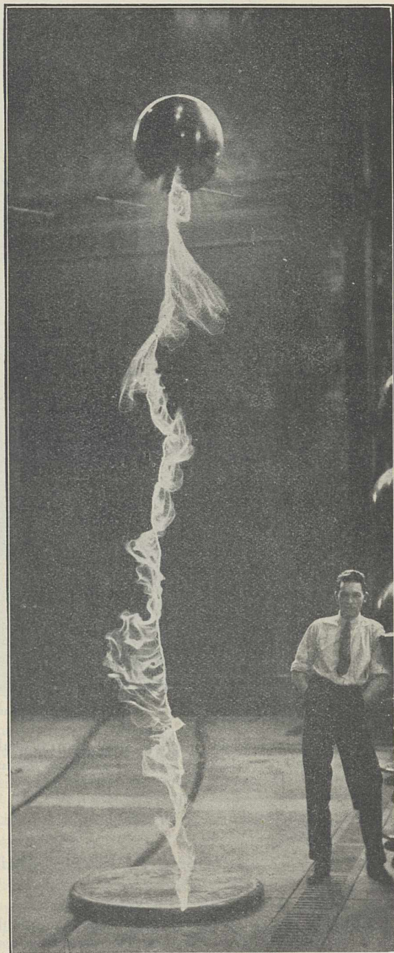
FIG. 2.—Power frequency arc at a pressure of 970,000 volts in a 12-ft. gap. The man was photographed separately.
