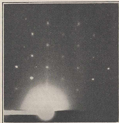
FIG. 1.—Diffraction pattern of cathode rays incident on a cube face of a single crystal of silver.
