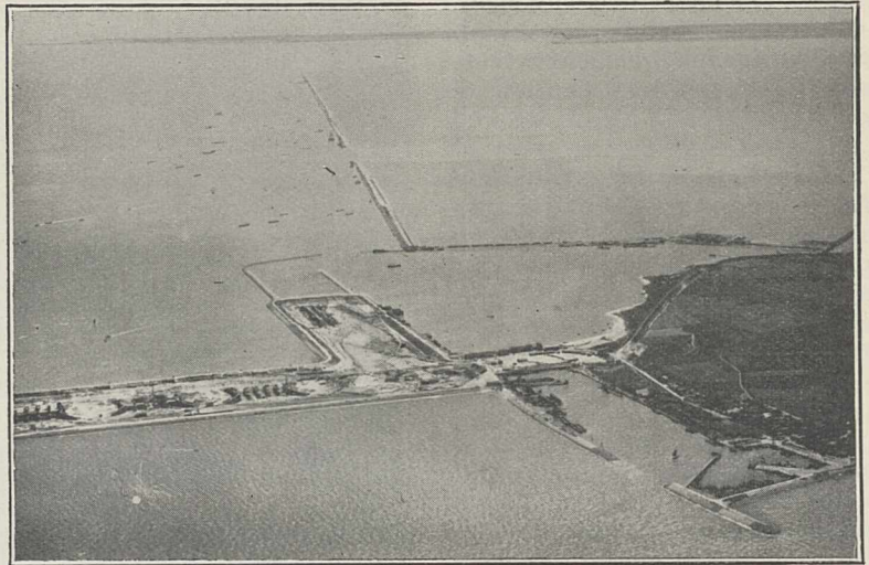
FIG. 2.—Aerial view at Den Oever showing main dyke extending to left, and in centre, dyke, enclosing North-West Polder, stretching towards Medemblyk on horizon. In the foreground, foundations for sluices and lock, with working depot and harbour.
