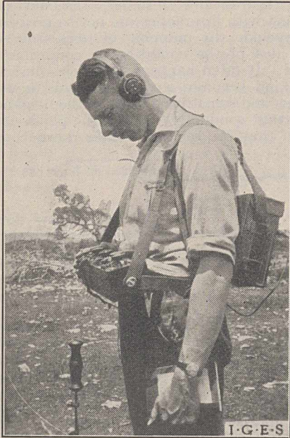
FIG. 3.—Ratiometer in use with amplifier on the operator's back.
