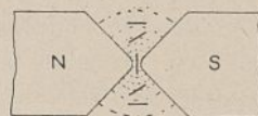
FIG. 9.—The black lines show different positions of a thin wafer of pressed bread hung by a single fibre. In the outer parts of the magnetic field it sets more or less along the lines, but as it is brought up to the more intense parts, where there is great divergence of the lines, it turns so as to set itself at right angles to the field.
