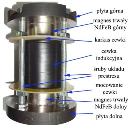
Rys. 8.20. Budowa harvestera TCCM (model 2) [116, 121, 122]
