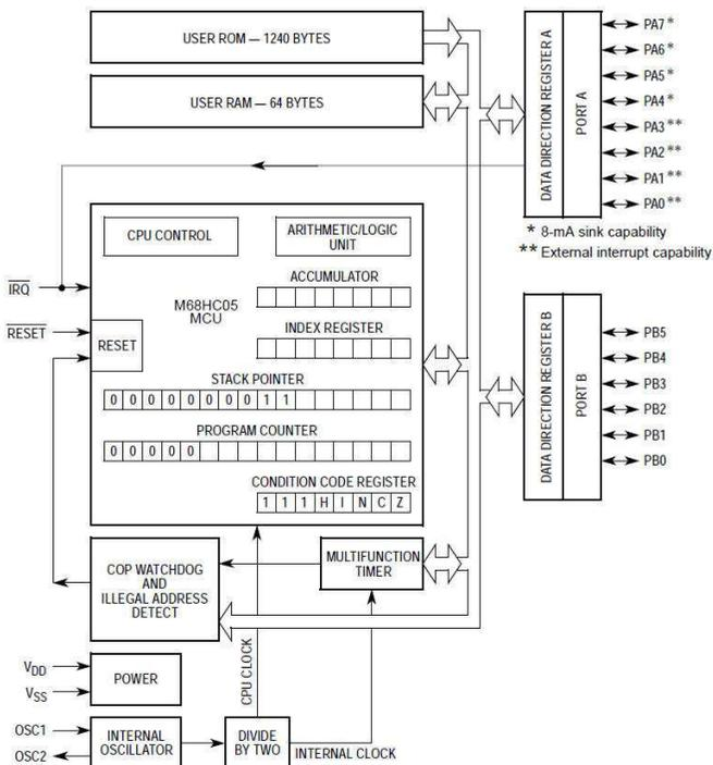
Figure 1.4. The internal diagram of MC68HC05J1A microcontroller (© Motorola/Freescale).
