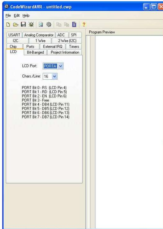
Figure 1.14. The recommended method of wiring for connecting LCD 16x2 display to Atmega16 microcontroller (suggestions given by CodeWizardAVR tool).
