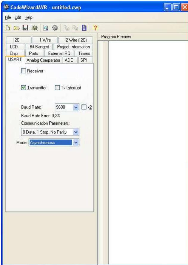
Figure 1.20. CodeWizardAVR window – USART configuration dialog
