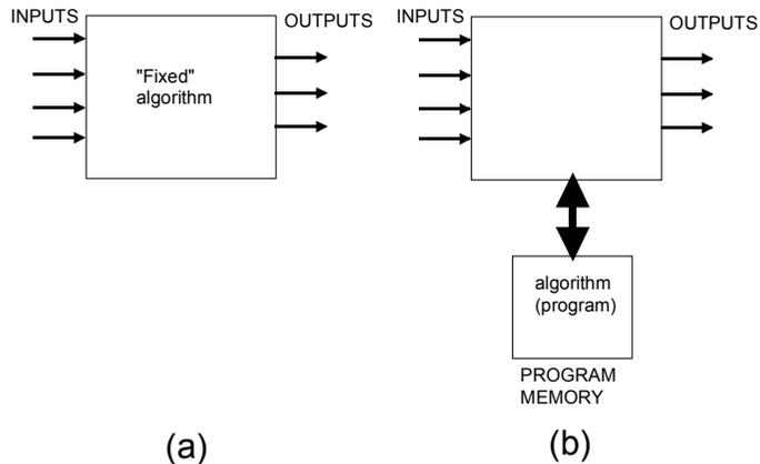
Figure 1.1. A comparison between a control system with a hardware fixed algorithm (a) and a programmable control system with an algorithm (program) located in an external memory (b).
