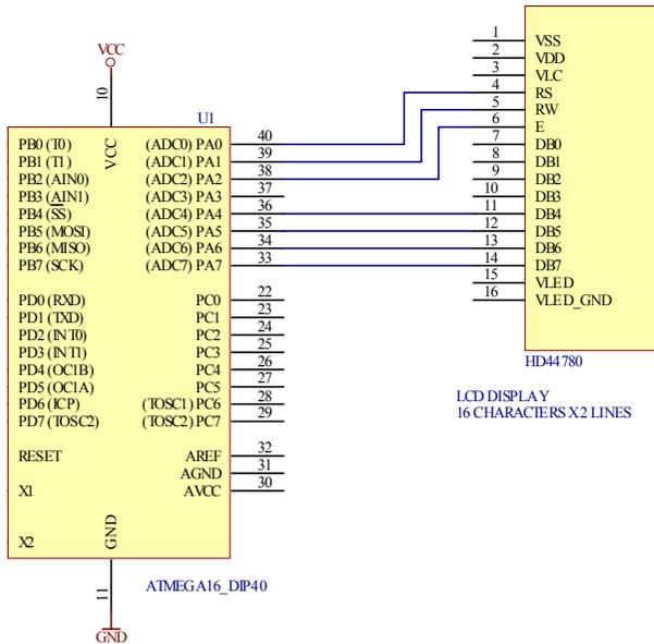
Figure 1.15. The wiring diagram for connecting LCD 16x2 display to atmega16 microcontroller.
