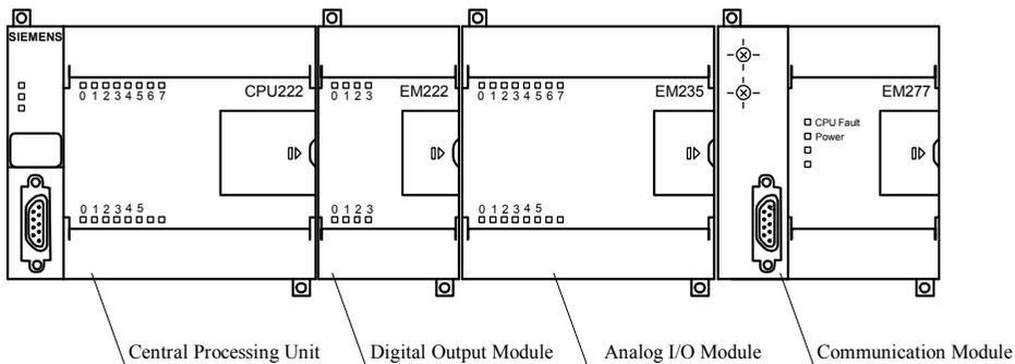
Fig. 2.1. An example of S7-200 hardware configuration
