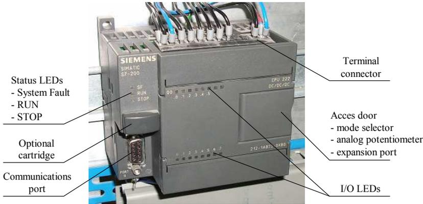
Fig. 2.2. S7-200 CPU: front panel, indicators, controls and connectors.
