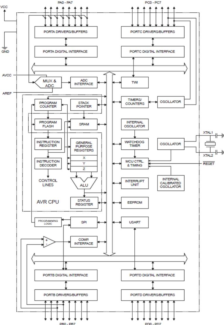
Figure 1.5. Atmel Atmega16 microcontroller block diagram (© Atmel)
