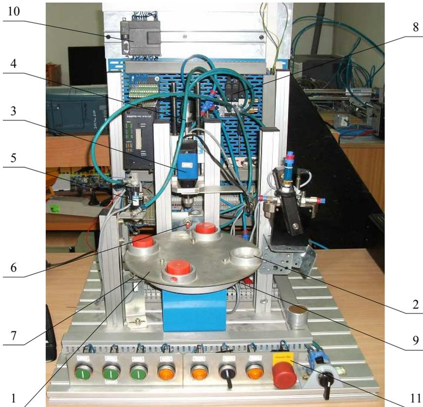
Fig. 2.6. The didactic station for rollers drilling process
