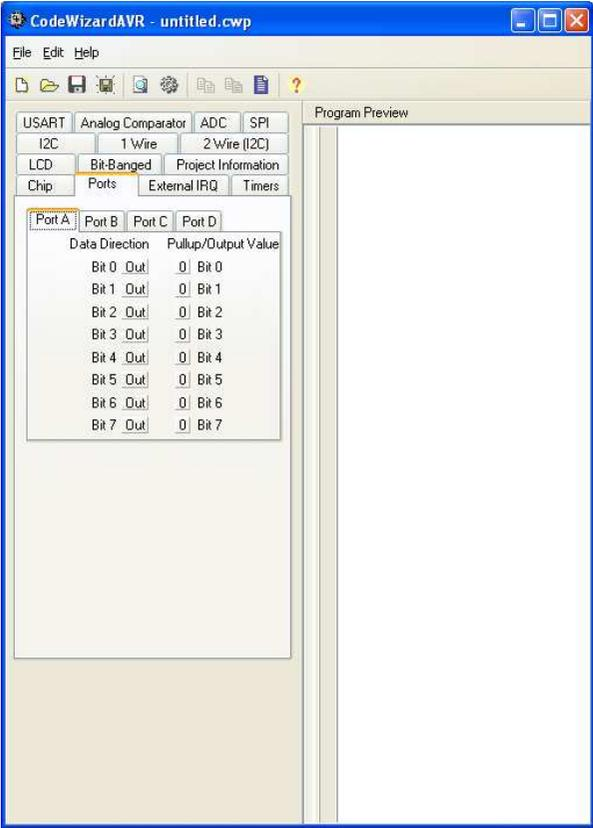
Figure 1.10. CodeWizardAVR window – I/O ports configuration dialog.
