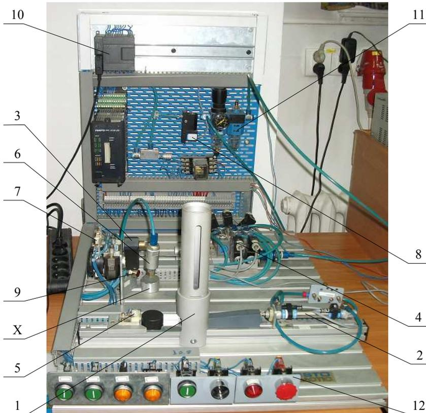
Fig. 2.4. The didactic station for rollers distribution process
