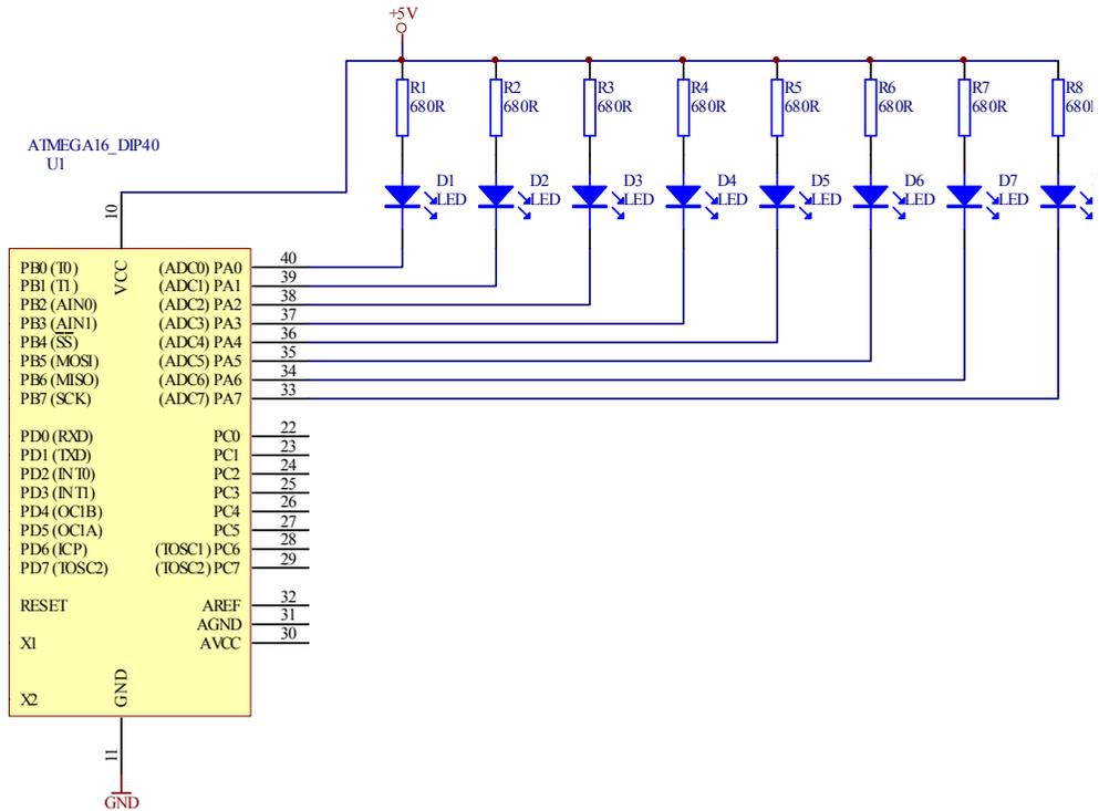
Figure 1.13. The wiring diagram for connecting LED diodes to the PORT A of an Atmega16 microcontroller.
