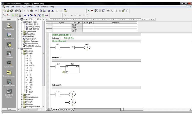
Fig. 2.3. An example of Step7-Micro/Win window with LDR editor
