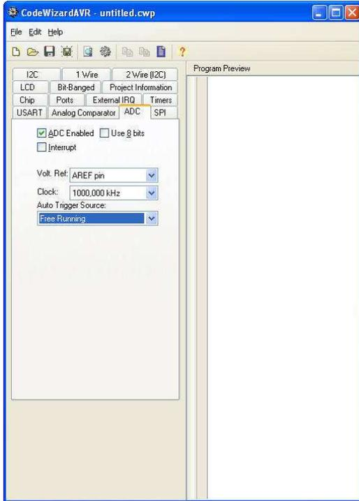
Figure 17. CodeWizardAVR window – ADC configuration dialog
