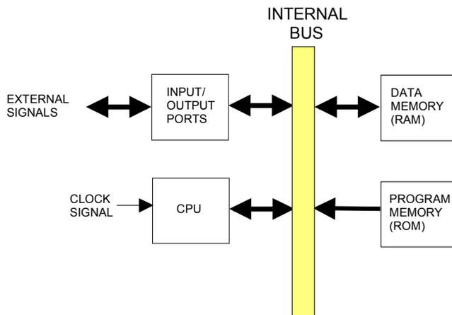
Figure 1.3. The general structure of a simple microcontroller. Please note the resemblance to the Turing machine.
