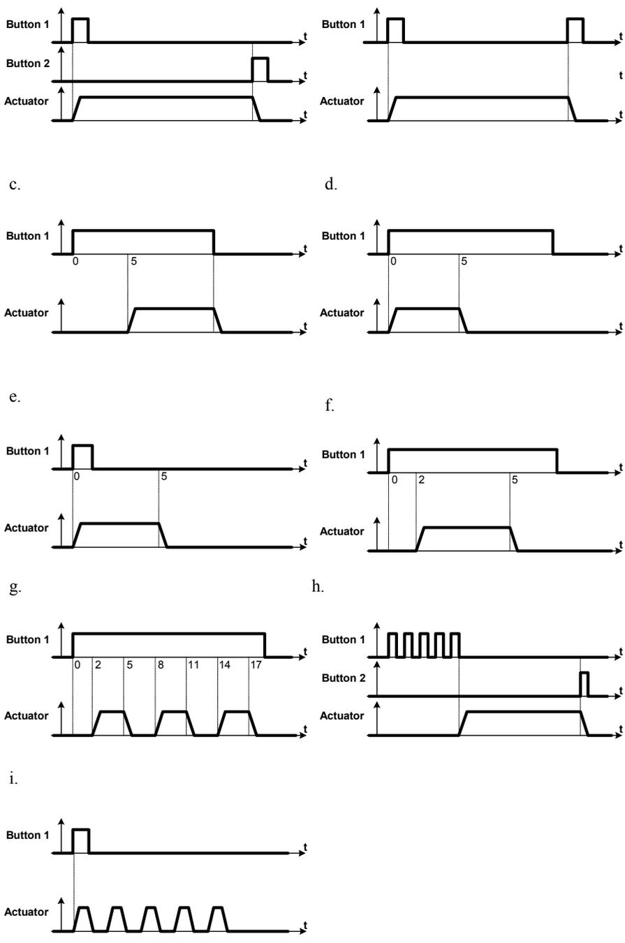
Fig. 2.8. Preliminary tasks – testing of Simatic’s fundamental functions
