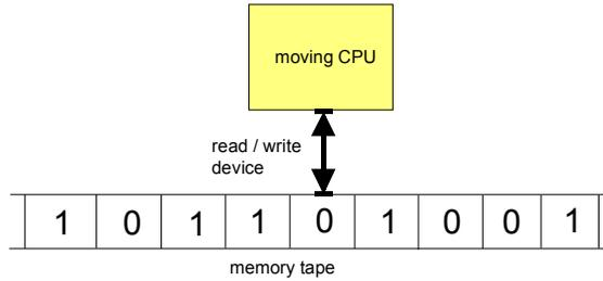
Figure 1.2. The general structure of the Turing machine. CPU= Central Processing Unit.
