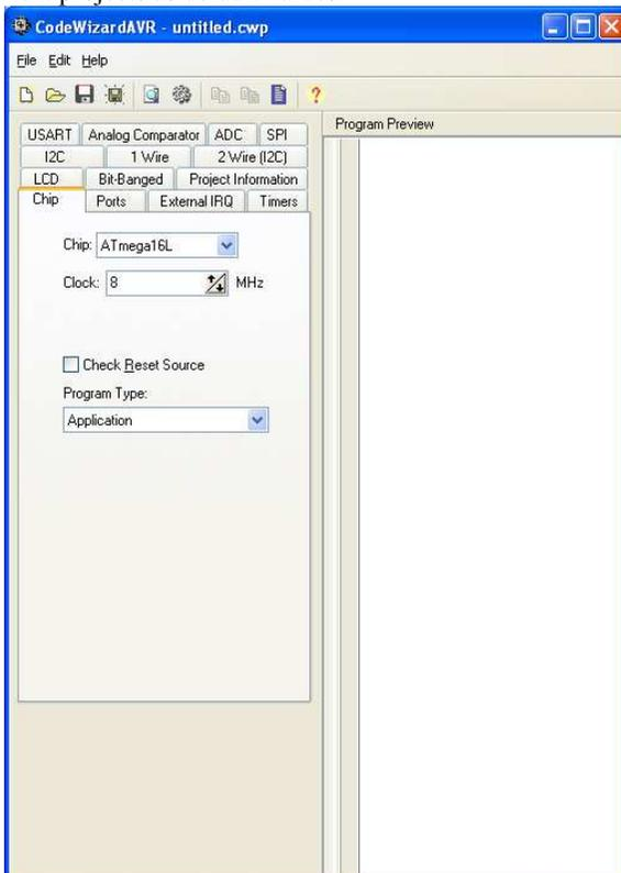
Figure 1.9. CodeWizard window – MCU type & clock speed selection.
