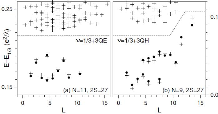
Fig. 10 The energy spectra of three quasielectrons (a) and three quasiholes in the Laughlin  $\nu=1/3$  state. The crosses correspond to the Fermi-liquid calculation using pseudopotentials from Fig. 8(a,b); the solid circles give exact spectra obtained in full diagonalization of the Coulomb interaction of eleven (a) and nine (b) electrons.
