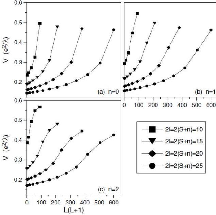
Fig7 The pseudopotentials  $V$  of the Coulomb interaction in the lowest (a), first excited (b), and second excited (c) Landau levels, calculated on a Haldane sphere, as a function of squared pair angular momentum  $L(L+1)$ . Different symbols correspond to different Landau level degeneracy  $2l+1$ .
