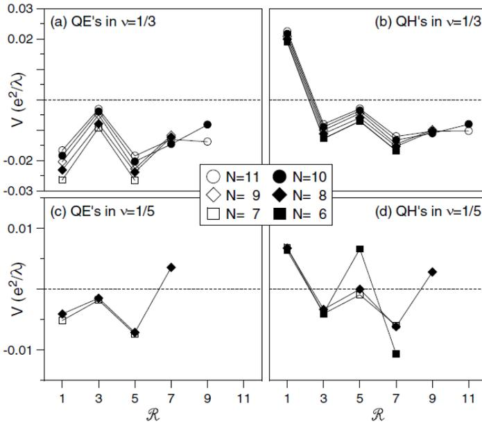
Fig. 8 The pseudopotentials of a pair of quasielectrons (left) and quasiholes (right) in Laughlin  $\nu=1/3$  (top) and  $\nu=1/5$  (bottom) states, as a function of relative pair angular momentum  $\mathcal{R}$ . Different symbols mark data obtained in the diagonalization of between six and eleven electrons.
