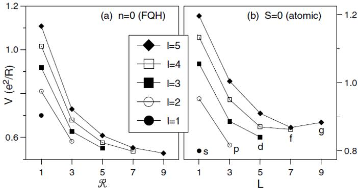
Fig. 5 The pseudopotentials  $V$  of the Coulomb interaction for the pair of electrons each with angular momentum  $l$ : (a) lowest Landau level on a Haldane sphere, monopole harmonics,  $n=0$ ,  $l=S$ ,  $V$  plotted as a function of relative pair angular momentum  $\mathcal{R}$ ; (b) atomic shell, spherical harmonics,  $S=0$ ,  $l=n$ ,  $V$  plotted as a function of pair angular momentum  $L$ .
