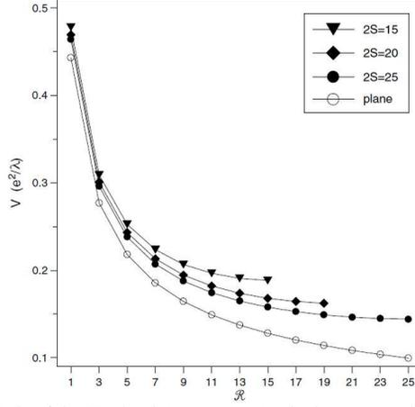
Fig. 3 The pseudopotentials of the Coulomb interaction in the lowest Landau level calculated on a Haldane sphere with  $2S=15, 20,$  and  $25$  (solid triangles, diamonds, and circles, respectively), and on a plane (open circles).
