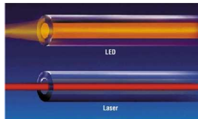
Fig. 3.5 Light beam emitted by a LED diode fills the volume of a multimode fiber core (top). A narrow beam emitted by a laser diode mostly propagates near the central part of the core (bottom) (DiMinico, 2001).
