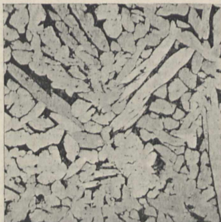
FIG. 2.—Micro-structure of alloy as cast in sand.
