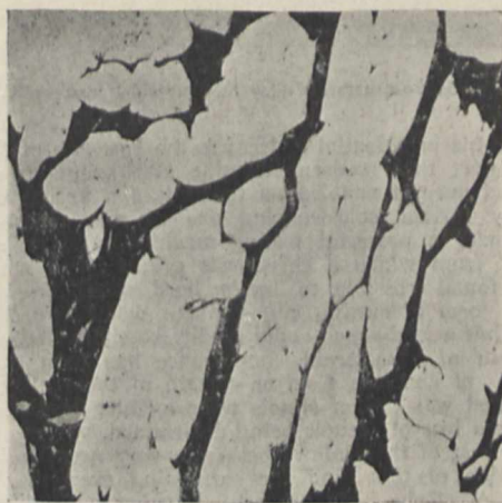
FIG. 3.—Micro-structure of alloy after long annealing at 900° C.
