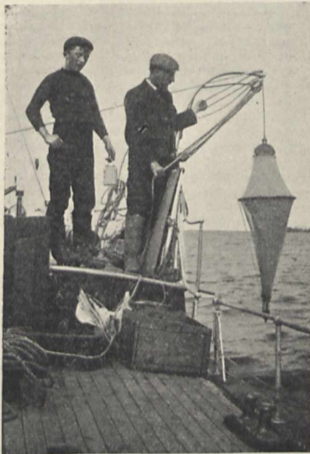
FIG. 4.—The Closing Petersen-Hensen Net going down open.
